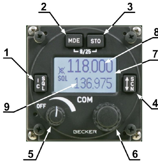
Fig. 11 Controls and indicators AR6201/GT6201
