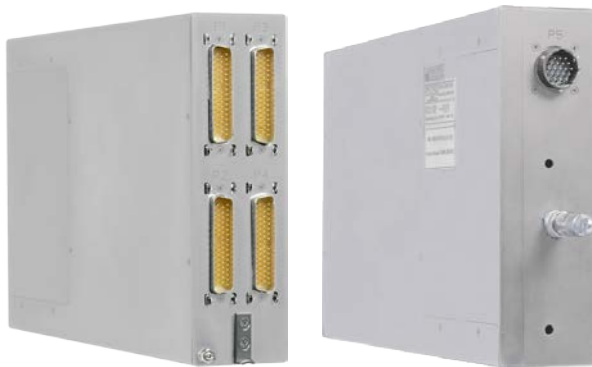
Remote Control Unit REU6100 (front- rear view)
