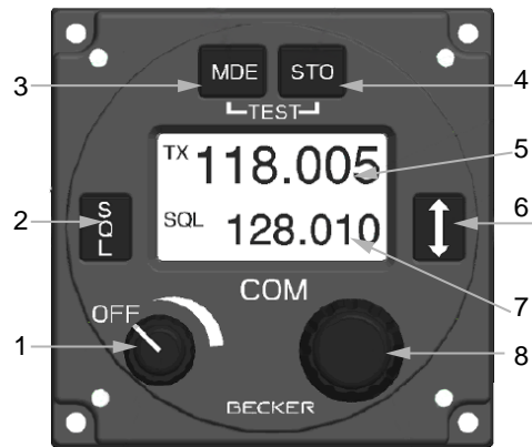
Figure 45: RCU6512 - Controls and Indications
